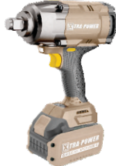
XPC-IW-07 BRUSHLESS IMPACT WRENCH 1800NM | M24-M42 | 6.0Ah
